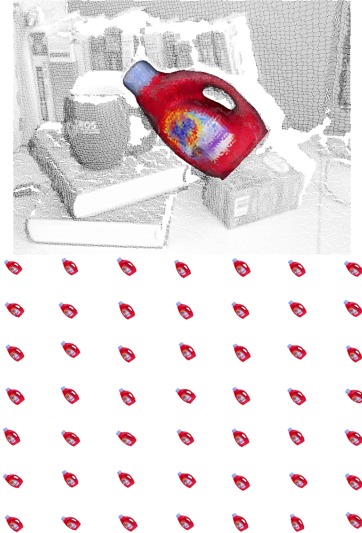
Figure 2.5.1: Example object tracking with the algorithm of Choi and Christensen. Multiple poses are rendered into one large texture (source: [CC13])
