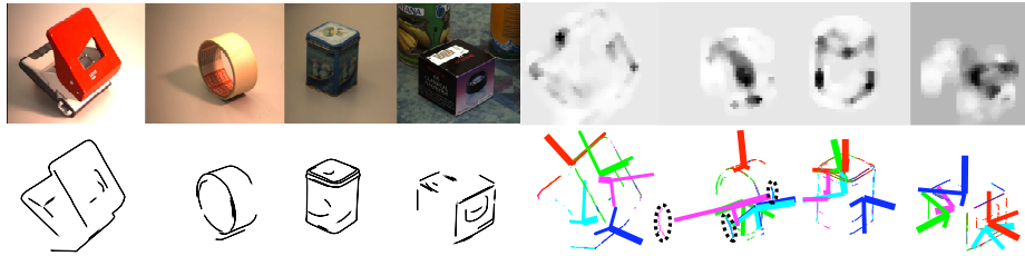
Fig. 4. Four objects, their matched contours, grasping point probabilities and finally the five best hypotheses for each object. The hypotheses are coloured, from best to worst, red, green, blue, cyan, magenta. False matches are circled in black. (Best viewed in colour)
