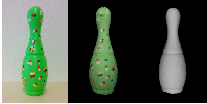
Figure 5.7: The bowling-pin object enriched with 2d texture using stickers (left). The added texture allows for the reconstruction of a reference ground truth shape (middle, right) facilitating quantitative evaluation.
