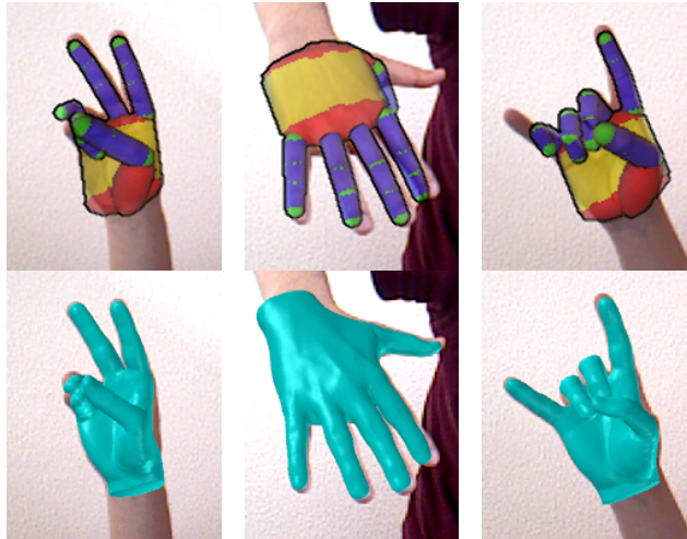
Figure 4.14: Qualitative comparison with [Oikonomidis et al., 2011a]. Each image pair corresponds to the pose estimate of the FORTH tracker (up) and our tracker (down)
