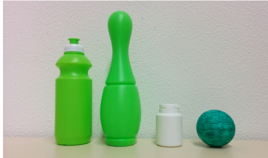
Figure 5.5: The objects to be reconstructed (left to right): a water-bottle , a bowling-pin , a small-bottle and a sphere . The dimensions of the objects are summarized in Table 5.1. All four objects are characterized by high symmetry and lack of distinctive geometrical and textural features, causing existing in-hand pipelines to fail. We perform successful reconstruction of all four objects.
