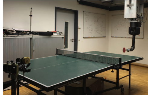
Fig. 1: The 7-DoF robot table tennis setup.
